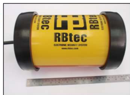
Under ground sealed capsule for local analyzer
