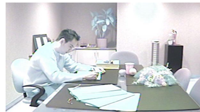
Conventional dual mode color / IR camera: Video taken without MFP technology suffers from IR bleed and poor quality color.
