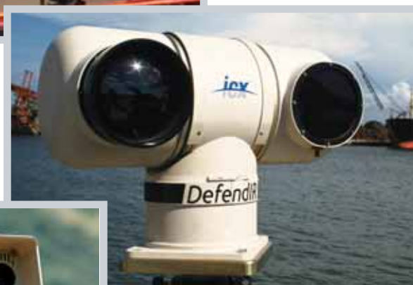
The Vindicator Radar Detection System uses thermal imaging products from various vendors including ICx Technologies and FLIR.
